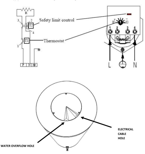
**IMPORTANT:** The electrical connections plastic cover on the side of the water tank should be installed as shown in the drawing above. The smaller hole is for the overflow of any water leaking into the electrics cavity and should be placed at the lowest point of the cover. The electrical cable hole is larger to accommodate for the diameter of the cable and protective sheath.
