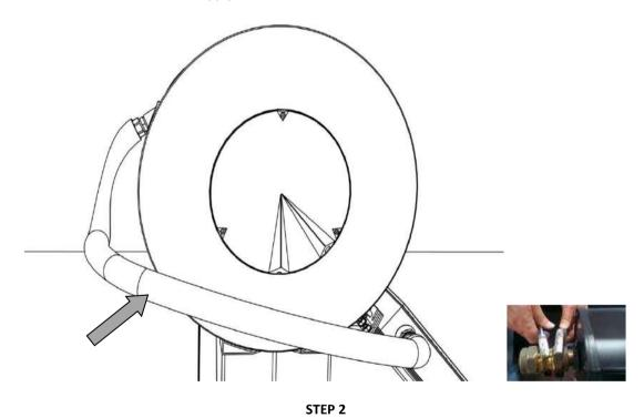
Connect the hot water closed circuit tube between the collector and the tank. Ensure that the tube follows an upwards route towards the tank. When tightening the fittings on the collector exit make sure you use 2 spanners, 1 for tightening and 1 against to avoid damaging the absorber.
