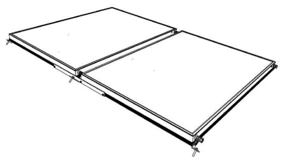
**Figure 1:** The two collectors ready for installation with top and bottom braces and collector feet installed.
