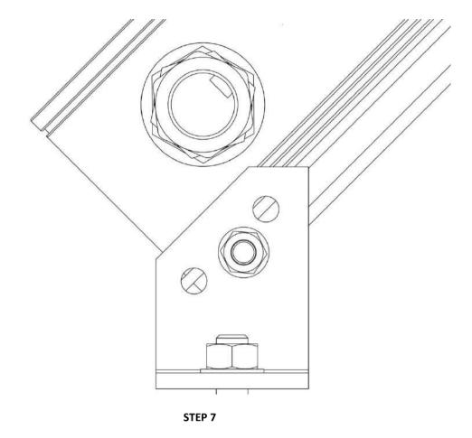
Ensure that the collector is set up to the appropriate angle. The collector support feet can be used as guides in setting the angle as they are cut at 45 degrees. The angle between the bolt, the bottom hole and the horizontal is 30 degrees. When the correct angle is set tighten all 8 bolts [4 collector bolts and 4 bolts at the bottom part of the support struts].
