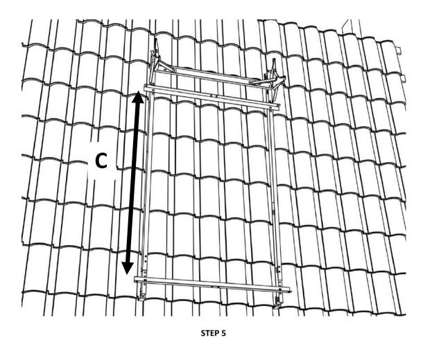
Install the two L beams supporting the collector. The distance C between the vertical mounting faces of two beams should be set according to Table 2 to fit the height of the collector. Secure only the bottom beam and slide the top beam upwards to ease collector installation.
