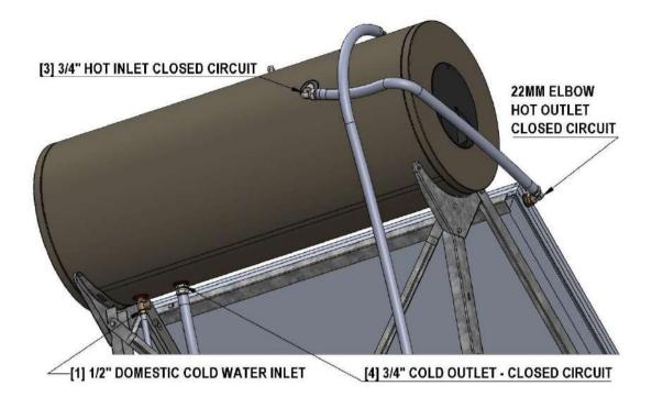
Figure 5: Thermosiphonic connection sizes.
