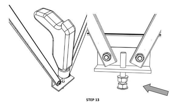
Using the hole of the brace foot as a guide drill the roof floor and install the securing bolt of the brace foot by tightening the bottom nut. Use fasteners of appropriate length and type to ensure that the collector feet are secured onto the structural layer of the roof and not on the insulation. **The fastener must protrude 7 cm** from the roof floor to allow for adjustments.
