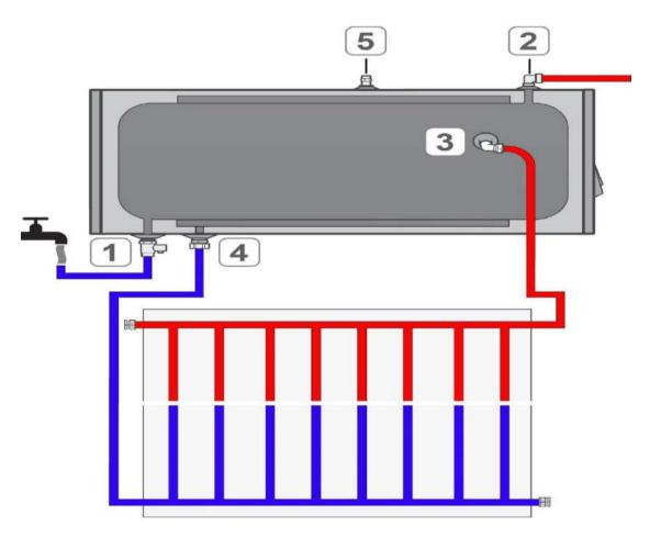
**Figure 4:** Thermosiphonic system layout and connections. [1] Domestic cold water supply, 10bar safety valve + non return valve. [2] Hot water outlet. [3] Closed circuit, hot inlet port. [4] Closed circuit, cold outlet. [5] 2.5 bar safety valve.
