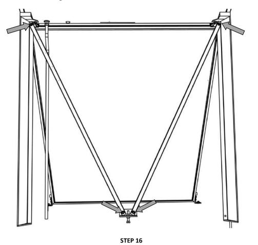
Tighten the 4 brace strut bolts. Make sure that all bolts are tight and that bolts are not loose on the base system.
