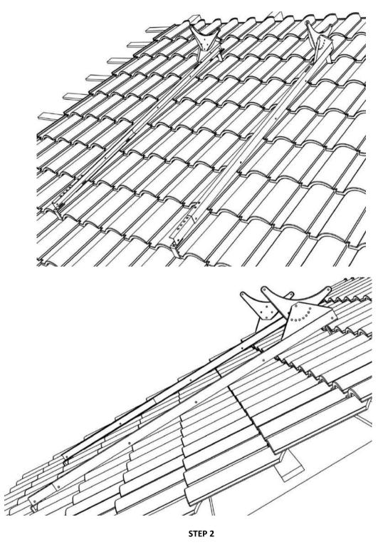
Replace the roof tiles and install the two longitudinal base sections onto the AGG brackets. Make use of the telescopic feature of the sections to adjust them to the appropriate length.
