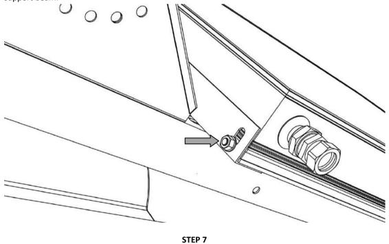
Slide the top support beam against the collector and tighten the support bolts. Tighten the support beam onto the longitudinal base sections.
