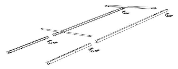
Figure 1: Components of the inclined roof base system.
