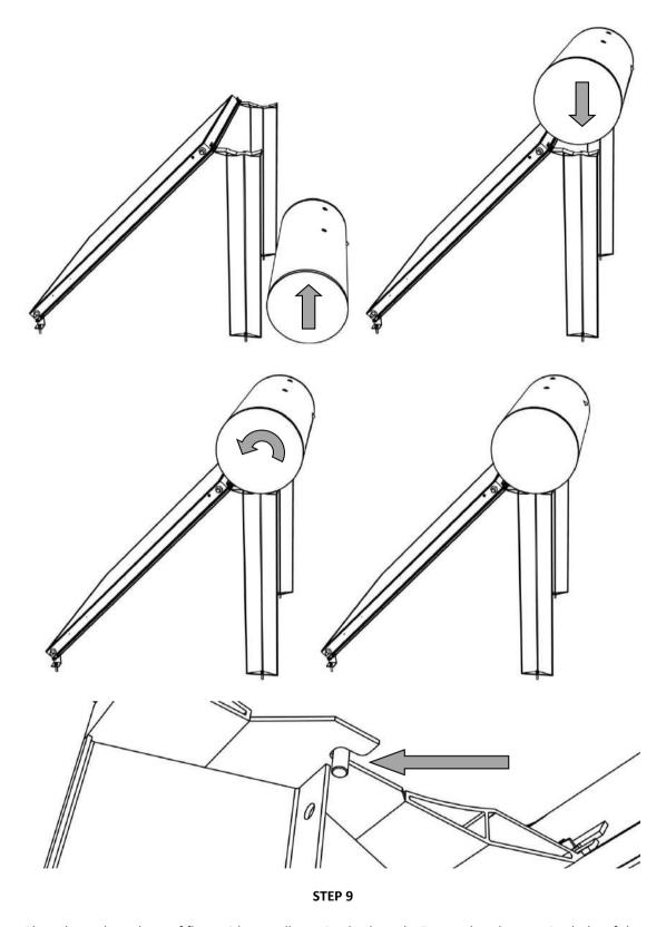
Place the tank on the roof floor with a small rotation backwards. Ensure that the securing bolts of the tank do not touch the floor. Lift the tank and place it on the circular seats on top of the pillars. Rotate the tank so that the tank securing bolts are inserted into the pillar slots.
