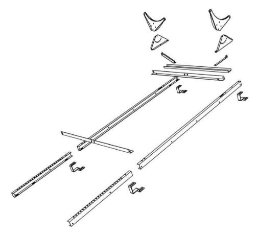
Figure 1: Components of the inclined roof base system.
