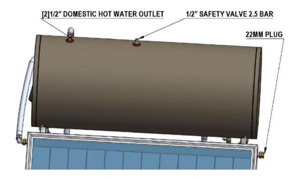
**Figure 6:** Thermosiphonic connection sizes. System shown is not MK5, however the connection are identical.
