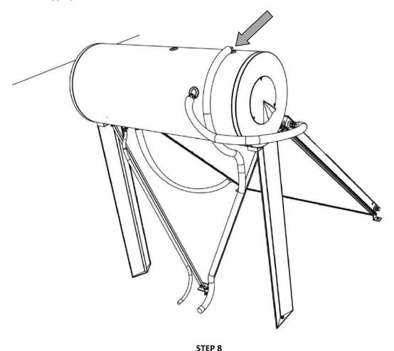
Connect the domestic hot water tube. Turn on the domestic cold water supply and check for leaks. The domestic water pressure should cause the closed circuit solution to overflow from the safety valve outlet at the top of the tank. If there is no overflow perform the diagnostic tests of Step 7.
