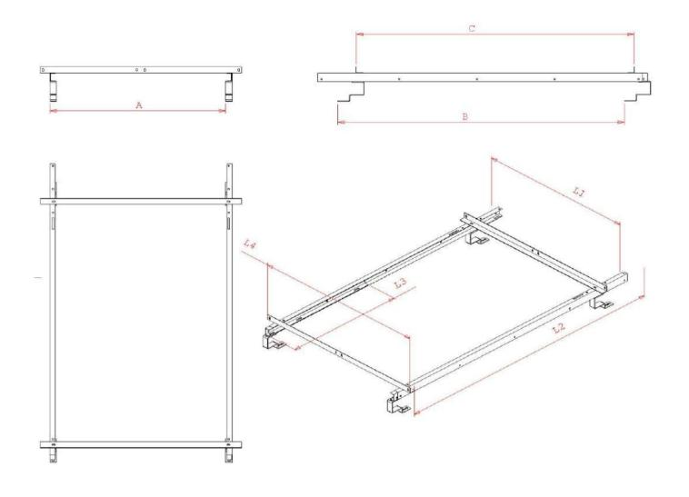
Figure 2: Installation and base system dimensions.
