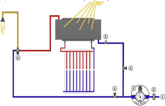
**Figure 3:** Schematic of complete system. [1] Domestic cold water supply according to DIN EN 806 or to country-specific regulations. [2] Water filter. [3] Pressure reduction valve MAX 10 bar. [4] Cut off valve. [5] Non return valve + 10 bar safety valve. [6] Cold/hot mixer for domestic hot water use, e.g. shower.
